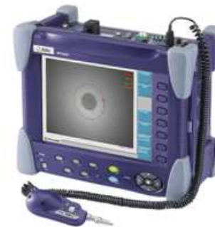
Microscope probe on the measuring instrument in the field
